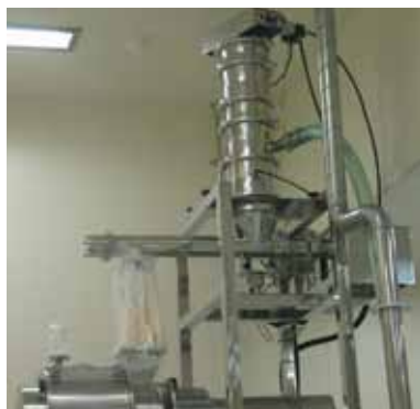
An example of Piab installation for powder transfer.
